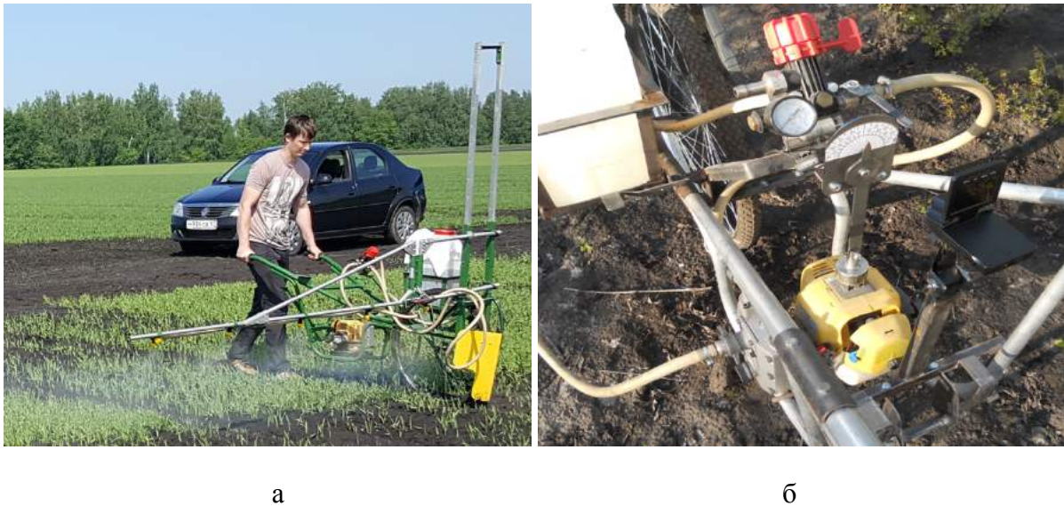
Figure 1: A prototype of a single-support boom motor sprayer (a) and a device for measuring the magnitude of horizontal deviations of the field boom (b)
