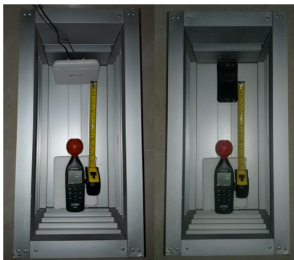
Figure 7: Photograph of aluminum box with measuring equipment and a. Broadband or wifi equipment, b. Cellular telephone equipment. Broadband or wifi equipment, b. cellular telephony equipment.
