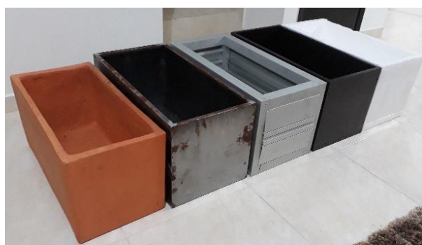
Figure 6: Photograph of simulation model boxes made of clay, metal, aluminum, melanin and icopor.
