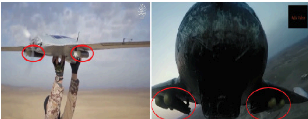
Image 3: Fixed-wing munition-loaded drone
