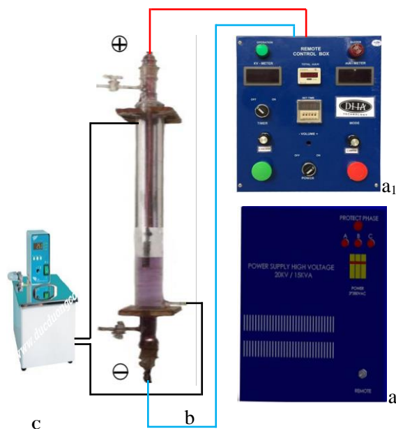
Figure 2: Model of DC high voltage equipment
