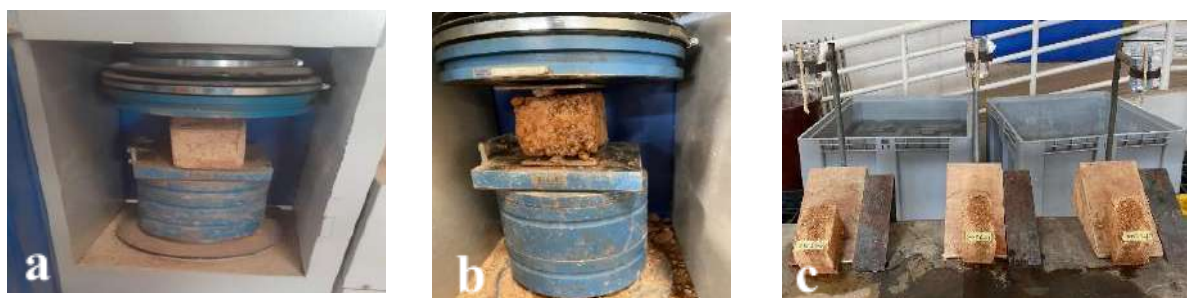
Fig. 3: Testing of CEB specimens: (a) compressive strength, (b) tensile strength, (c) erosion test
