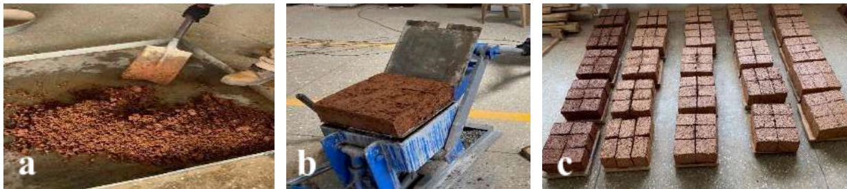
Fig. 2: Preparation of CEBs: (a) mixing of mortar, (b) moulding of blocks, (c) curing of blocks
