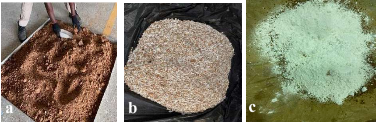
Fig. 1: Sample raw materials: (a) earth sample, (b) crushed eggshell samples, (c) lime sample
