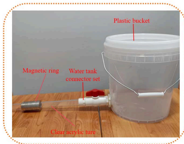
Figure 1: Physical diagram of self-contained pipe plug simulation device
